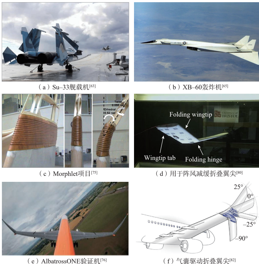
图8 折叠机翼与折叠翼尖设计方案 Fig.8 Design scheme of folding wings and folding wingtips
