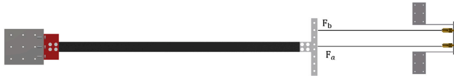
Fig. 9. Elevated view of the test configuration and the pulling forces applied to the tip fixture.
