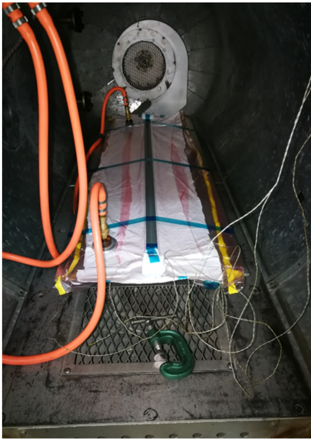
Fig. 3. The vacuum bagged beam inside the autoclave.
