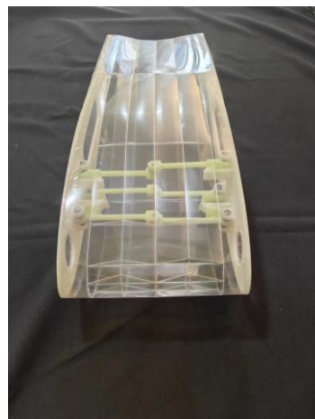
Figure 13. The spanwise morphing wing unit model.
